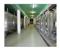
After the settling of the juices, the alcoholic fermentations are conducted in thermoregulated stainless steel tanks: a maximum temperature of 17°C is maintained to preserve the fruity aromas of the wine.
